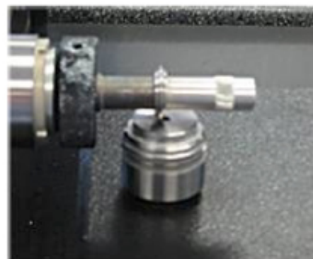
Figure 1: Schematic drawing at left showing the offset position of the dimpling tool. The image at right shows the configuration of the tool and platen during the initial phase of the alignment process.
